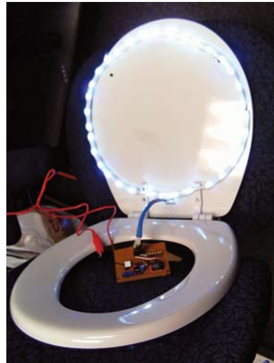
UV light is attached to the seat cover of this prototype; it will kill germs while the seat is down. The light will shut off as soon as the cover is lifted.
